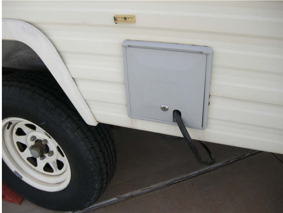
Photo of Electrical connection door, located aft of the wheels on the street side of trailer
