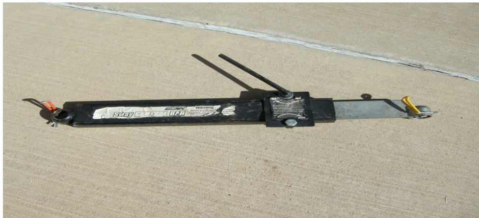
Photo showing Sway bar assembly.
