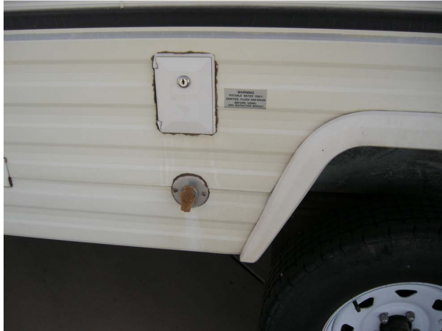
Photo of water connection door located forward of wheels on street side of trailer.
