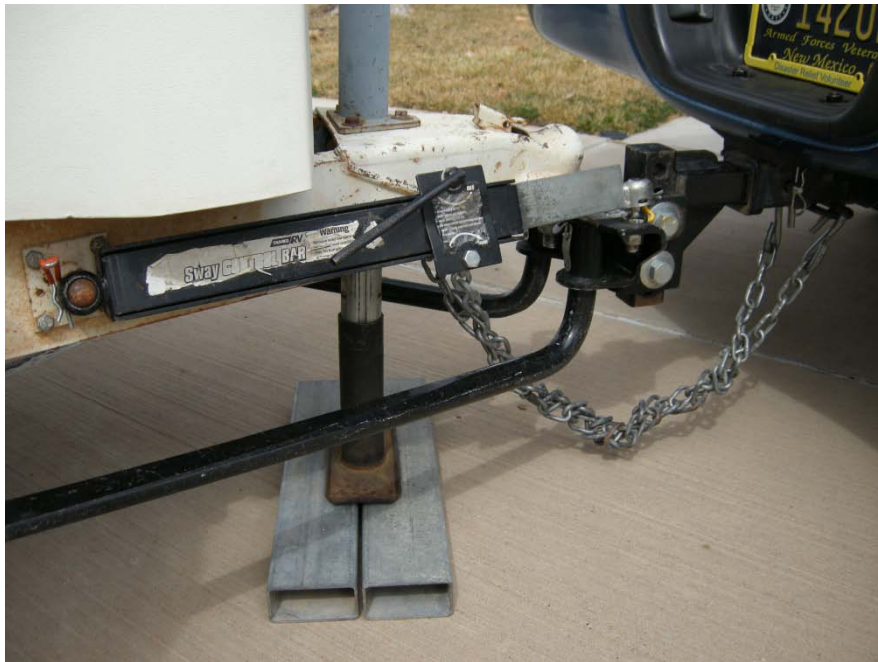
Photo of Sway bar installed.
