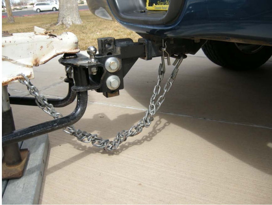
Photo of equalizer receiver installed
