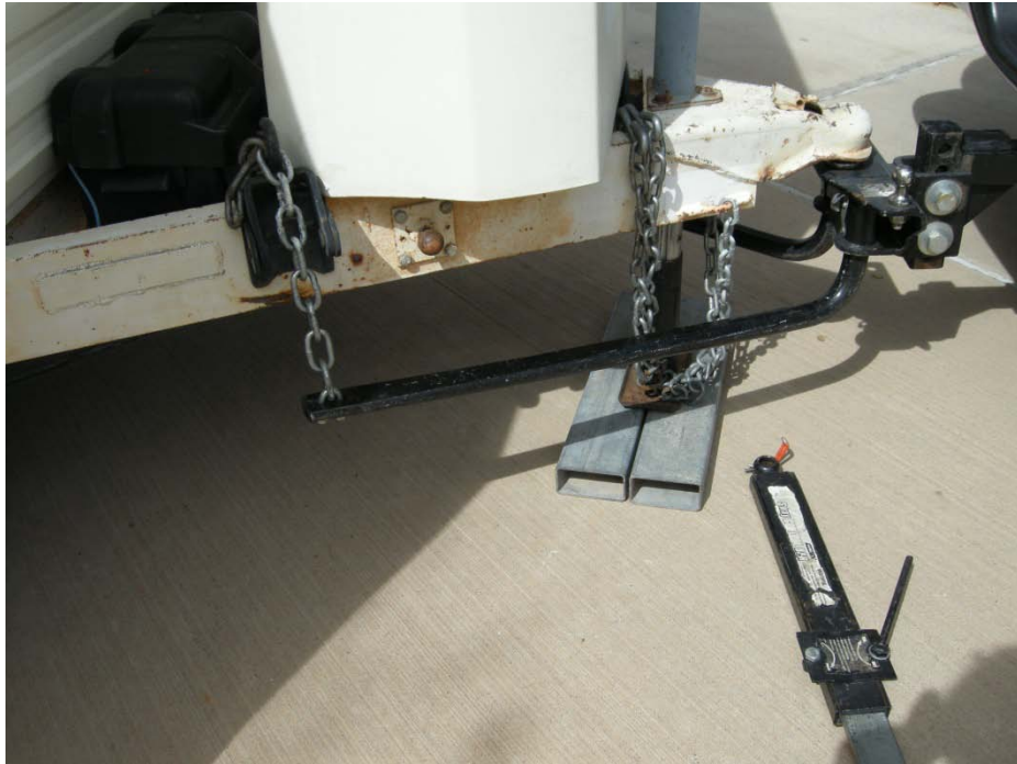
Photo of equalizer installed, one bare located on each side of hitch assembly.
