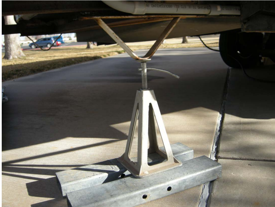
Photo of Stabilizer jack installed, position one at each of the four corners of the trailer.
